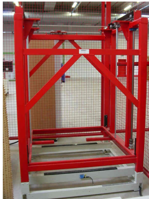
Separate stack lifting cage in parking position
