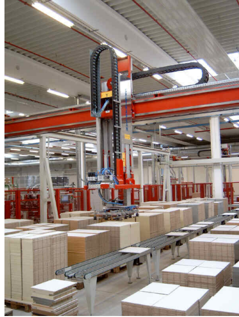
Area storage with direct transport connexion to following machines
