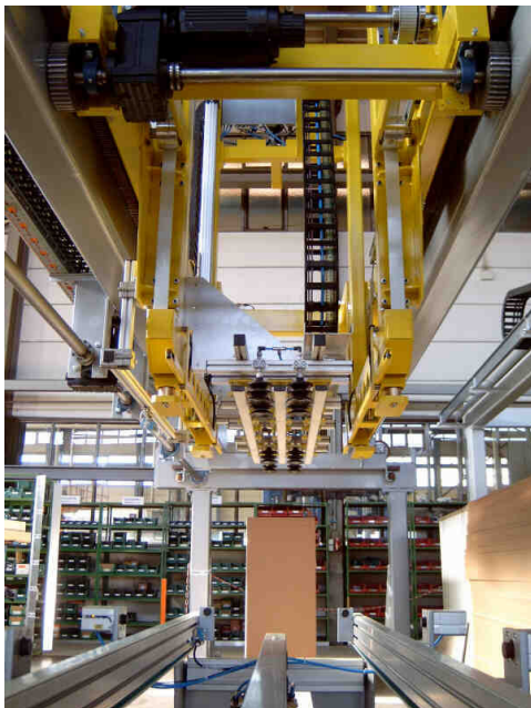
Fix installed stack lifting cage with suction frame
