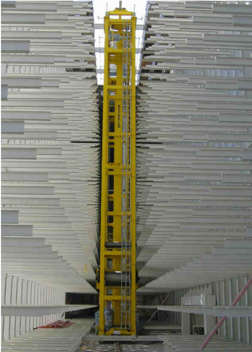
Automatic storage and commissioning system for flat materials with two independent working lifting platforms
